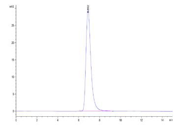
The purity of Biotinylated Human IL-18 R1 is greater than 95% as determined by SEC-HPLC.
